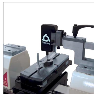
Calibration of small plain ring gauges (TA-SU-313, TA-MS-370, TEL76, TA-SU-354)
