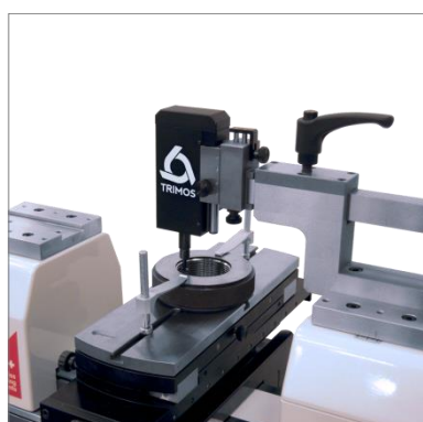
Calibration of threaded ring gauges (TA-SU-313, TA-MS-370, TA-SU-354, TUML13.2, TA-MS-307)
