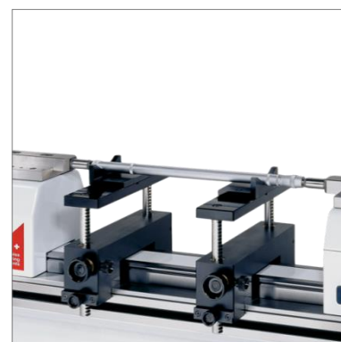
Calibration of 2-point internal micrometers (HPA-1, TELMA7, TELMN7.2)
